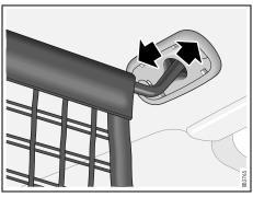
Attaching the cargo net to the roof
