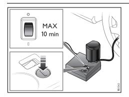
If the correct pressure is not reached within 10 minutes, the damage to the tire is too large to be repaired with the sealant. Park the car in a suitable place and call for assistance.
