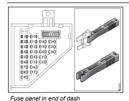
Some fuses and relays may be fitted but not connected to the car's electrical system.
