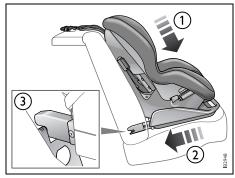
Rigid 2-point lower anchorage with top tether
