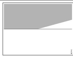
Correctly adjusted low beam
