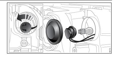
it locks. To facilitate fitting, look in through the headlight lens when fitting the bulb. Check that the new bulb is firmly seated.
