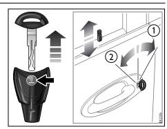
Locking/unlocking the front left-hand door with the traditional key
