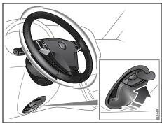
Lever for steering wheel adjustment
