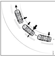
The illustration shows how the system brakes one or more wheels (and with varying braking force for each wheel) in order to increase the car's chances of following the direction in which the driver wants to drive.
