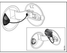
When refueling, hang the fuel cap inside the fuel door
