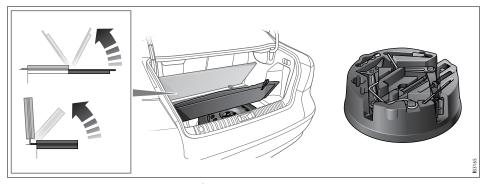
The spare tire, the tools and the jack \* with its crank are carried under a panel in the trunk.
