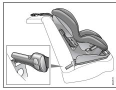
Semi-rigid 2-point lower anchorage with top tether
