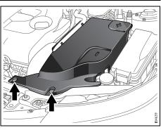
Turn the two retainers a quarter turn to unlock the battery cover.
