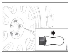
Removing the plastic wheel bolt covers
