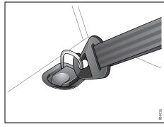
Cargo net fitted in front anchorage eye
