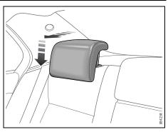
• Lowering the rear head restraints: press the head restraint forward and downward.
