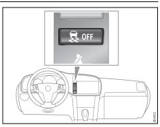
ON/OFF switch for ESP
