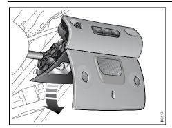
Hatch opened for replacement of center bulb
