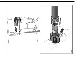
There are four adapters on the underside of the compressor which allow the compressor to be used to inflate other items such as bicycle tires, air mattresses and footballs.
