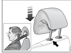
The front and rear head restraints can be raised and lowered to a number of positions.
